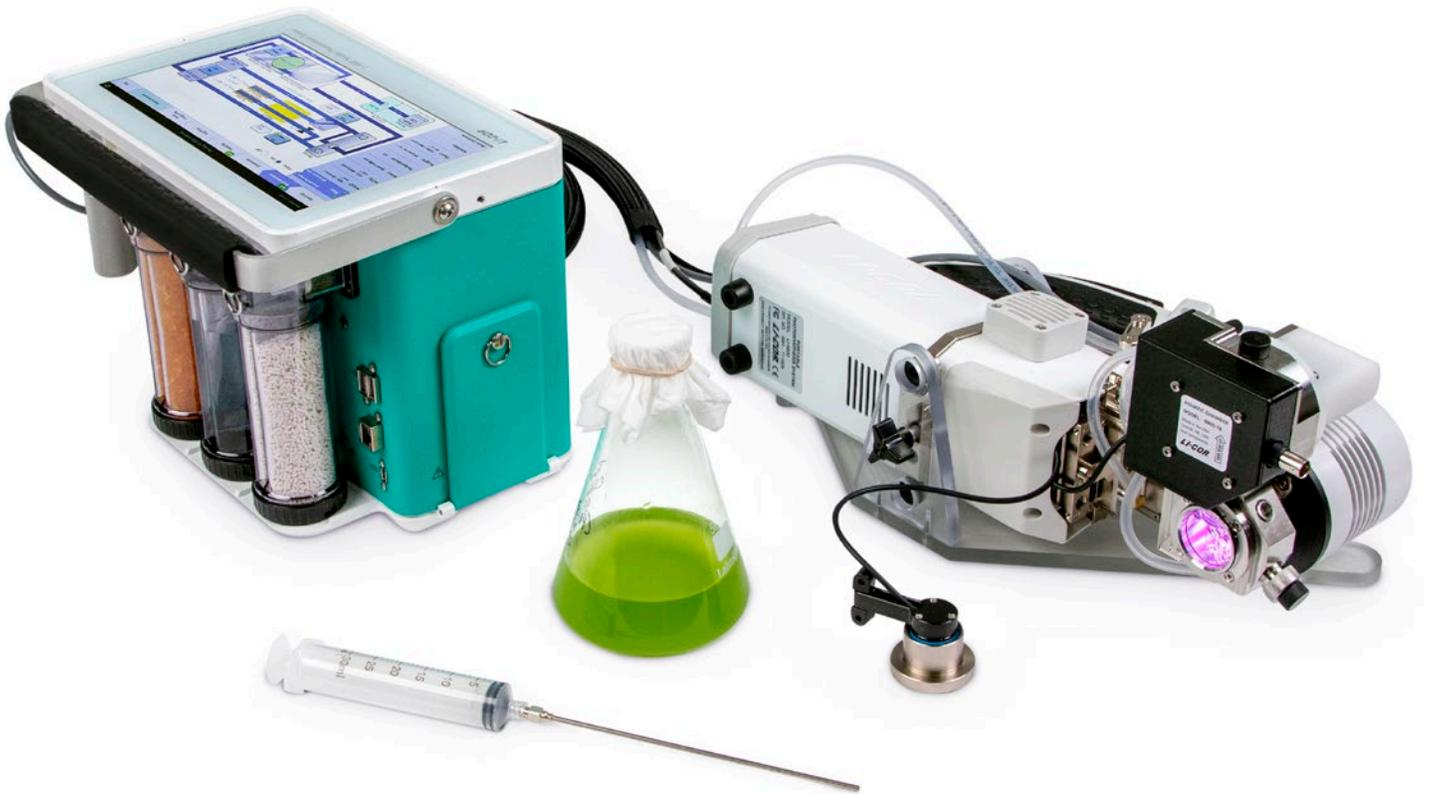
The Aquatic Chamber (6800-18) provides measurements of CO<sub>2</sub> exchange and chlorophyll *a* fluorescence from samples in liquid water, such as algal suspensions, or samples that require high ambient humidity, such as bryophytes. Assimilation is computed from the concentration differences and flow rate
