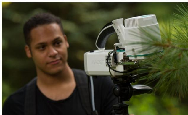
The Large Leaf and Needle Chamber (6800-13) is compatible with the large light source.
