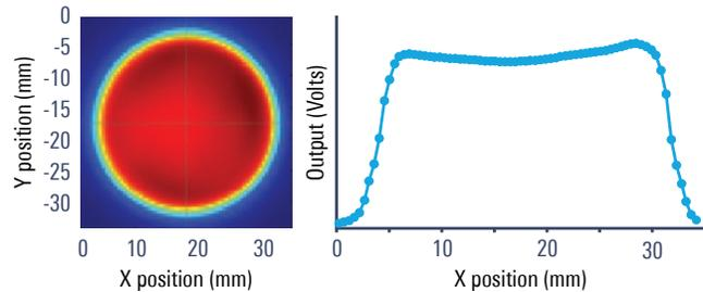
Figure 1. The 6800-01A Fluorometer provides uniform illumination, with light intensities within  $\pm 10\%$  of the mean over 90% of the leaf area.
