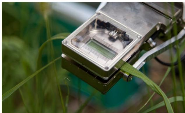
The Clear-top Chamber (6800-12A) is compatible with the small light source.
